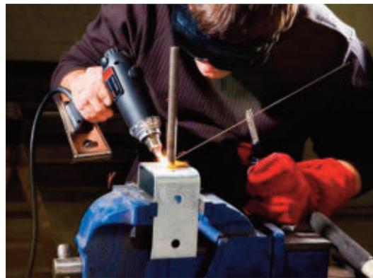
The Multiplaz 3500 power source can be used for welding and cutting jobs and requires no gases for either application. It requires only a tailored 8-oz. mixture of alcohol and water to help generate a plasma flame for welding and requires only 8 oz. of water to generate a cutting flame.
