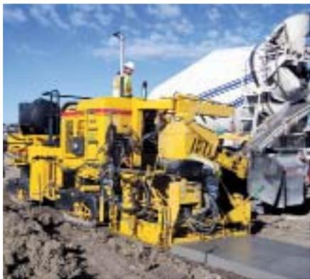
The GT-3200 sidewalk paver can be equipped with a front-mounted adjustable aggregate base mold to spread base aggregate for a sidewalk. The paver has a 20-in.-wide, 14-ft-long folding conveyor. The conveyor allows ready-mix trucks to discharge from the street instead of driving over curbs to reach the paver. The paver also features all-track steering.
