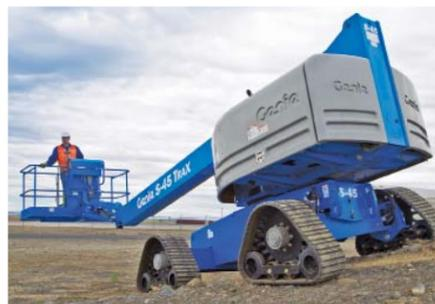
Genie S-40 and S-45 telescopic booms use the "four-point" Trax track drive system that reduces damage to sensitive ground surfaces. The S40 Trax has a lift
