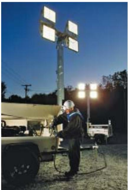
The ShorePlug connector, standard on all new AL4L generator LED light towers, allows multiple light towers to be connected in-line and operate from a single power source. LED light towers offer crisper lighting capabilities and consume less electrical power. The ShorePlug connector makes it quick and easy to take advantage of the power efficiency of LED lights by safely and securely connecting multiple towers in-line to operate from a single generator, reducing fuel consumption and engine noise.
