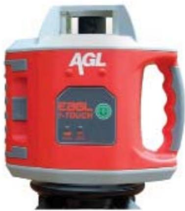
The EAGL 1-Touch is suitable for checking and setting elevations, forms, and footings; subbase leveling; and for visual and automatic machine-control applications. High-performance tilt sensors ensure precise, repeatable self-leveling of better than  $+1/16$  in. at 100 ft.
