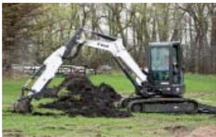
The M-Series E55 compact excavator comes with an extendable telescoping arm option for an additional 30 in. of reach when fully extended. When retracted, it delivers similar tear-out force as a standard arm. It's also the first extendable arm for a compact excavator that allows the use of a hydraulic clamp, for picking up and placing materials, such as rocks, landscaping materials, and debris. It's controlled via a rocker-style thumb switch on the joystick.
