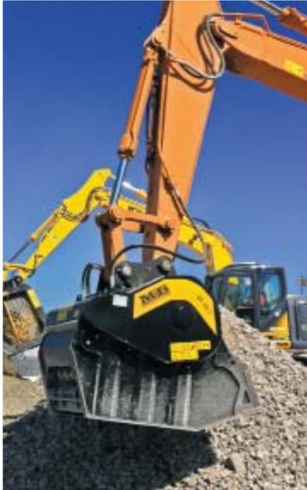
Attach the Crusher Bucket to an excavator to crush reinforced concrete and other material right in the bucket, eliminating the need to haul waste to a dump by returning clean rebar and material that's ready to be reused. Four models fit excavators 9 tons and larger.
