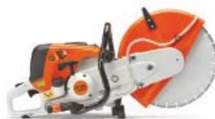
TS 410 A (EWC) Cutquik Cutoff Machines offer control over water flow to the cutting surface. The EWC stops the water flow at idle speeds and automatically starts again when the throttle is fully engaged. Offers an anti-vibration system, mounted keypad, and an X2 low-maintenance air filter system.
