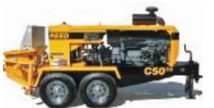
The C50SS concrete pump packs superior performance in a compact frame. It's designed for extreme long-distance pumping such as high-rises and tunnels, as well as high-volume shotcrete applications. It combines a 220-hp, 164-kW Cummins diesel and 180cc main hydraulic pump. It sports a maximum output of 54 cu yd/hr at 2000 psi concrete pressure.
